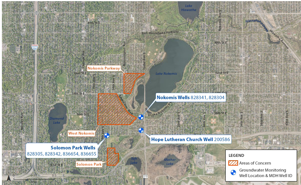
Figure 61. Groundwater Wells. Seven groundwater monitoring wells exist near the near the Areas of Concern. (Credit: MCWD)
