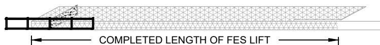
FIG 2. CONSTRUCT FES LIFTS ALONG LENGTH OF FIRST SET OF FORMS AND THEN BEGIN PLACEMENT OF FORMS AND CONSTRUCTION OF SECOND LIFT.
