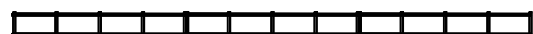
FIG 1. PLACE A ROW OF CONSTRUCTION FORMS ALONG DESIRED CHANNEL ALIGNMENT FOR FIRST FES LIFT.
