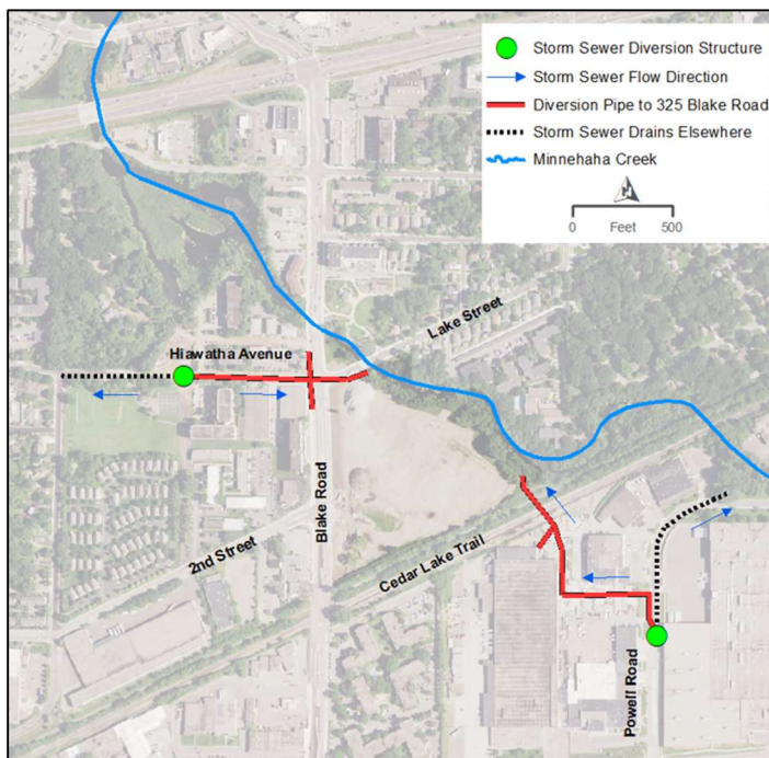
Figure 4.1: Storm Sewer Diversions. Stormwater collected from Powell Road and Lake Street is diverted to the site. When the diversions reach capacity, excess runoff discharges to separate locations.
