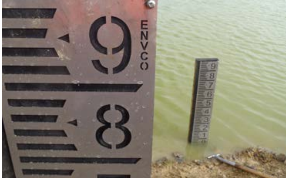
1 STAMPED METAL PANEL WITH WATER ELEVATION AND FLOW DIRECTIONS "IN" AND "OUT"
