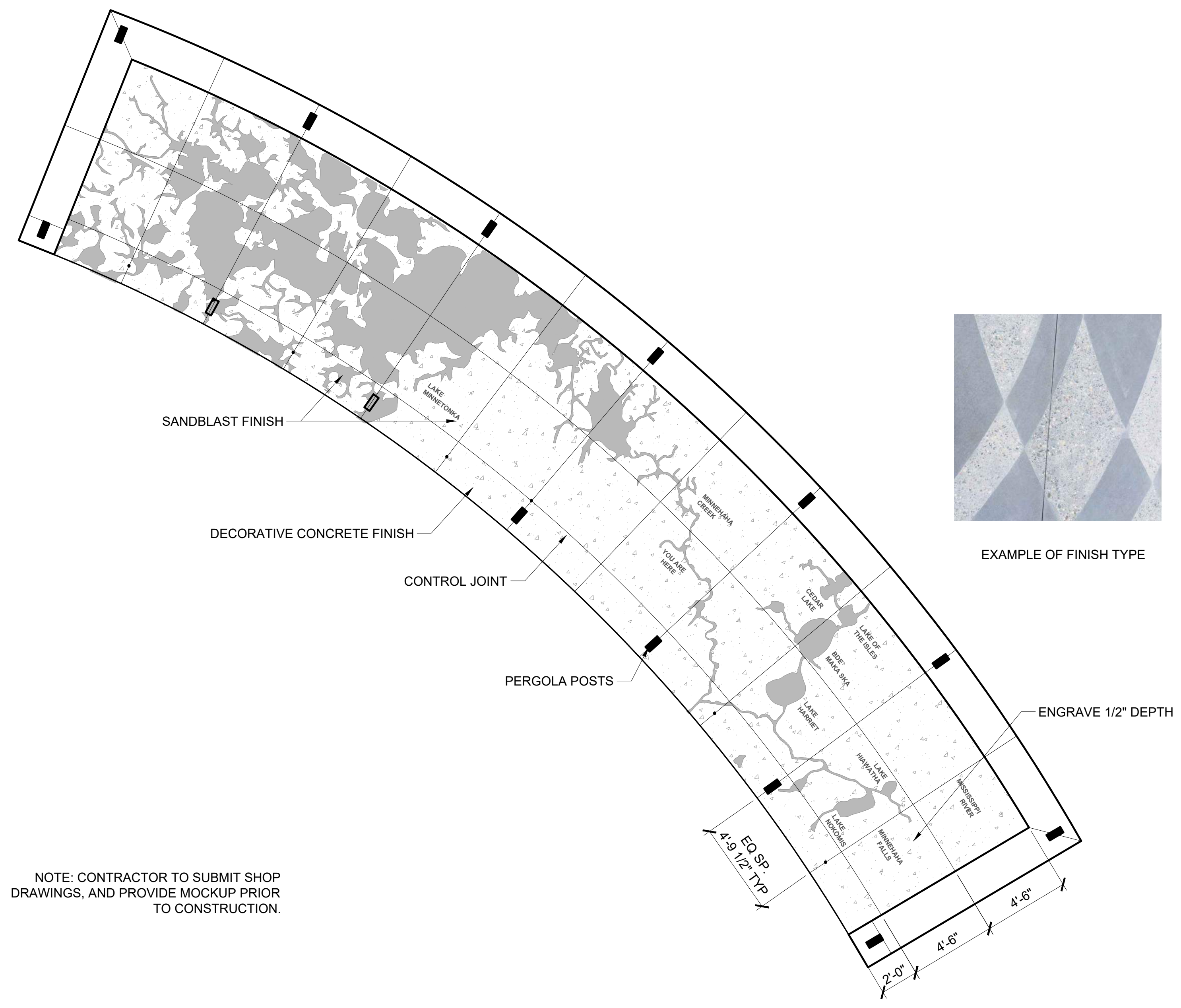
1 DETAIL-OVERLOOK PAVING PLAN (DEDUCT ALTERNATE) 1/4" = 1'-0"
