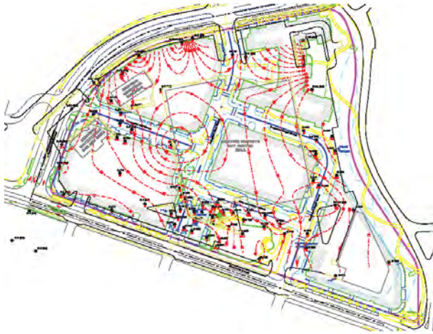
“Turbulent sea of hydrogeology” – wildly varying depth to sand contours (5’ intervals). AET, Inc.
