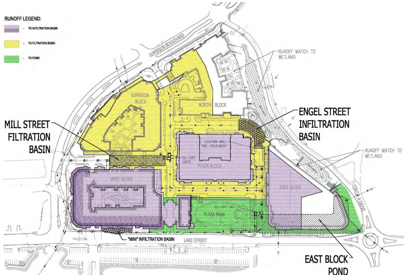
Primary stormwater systems at The Promenade of Wayzata: Engel Street Infiltration Basin, Mill Street Filtration Basin, East Block Pond. Runoff areas to each system are indicated in color according to the legend.
