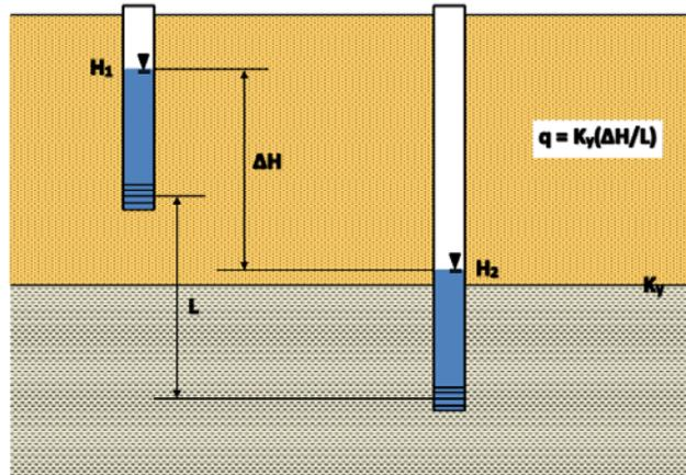
Figure A.11. Darcy flux approach used to calculate value effective  $k_v$  to supply 6.5 inches/yr leakage between the surficial and underlying Prairie du Chien aquifers in regions of the watershed where these aquifers are in direct contact.
