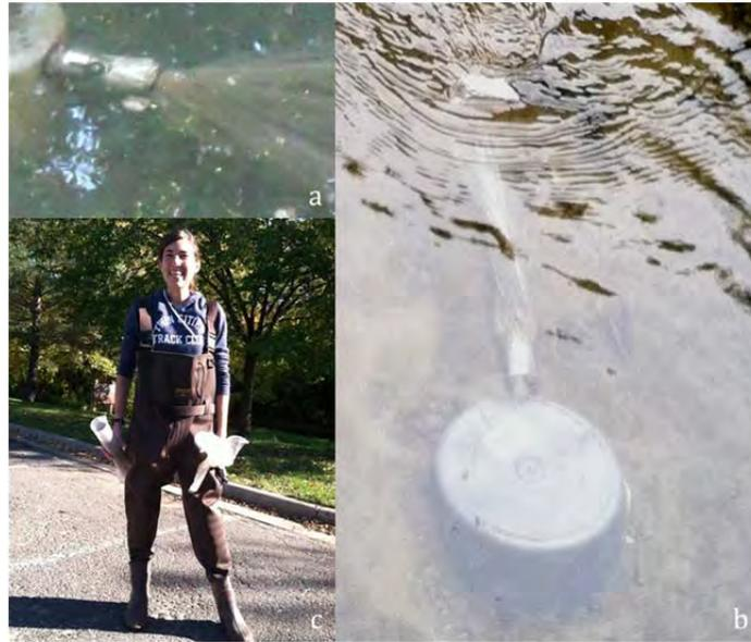
Figure 8. Seepage meters used to measure fluxes into or out of the streambed. (a) Close-up of hose-fittings used to attach the seepage meter to a plastic bag in which the change in volume of water over a set period of time is known. The valve is closed when the bag is being removed or being attached to avoid losing water. (b) Seepage meter deployed in streambed. (c) Measuring the volume of water in seepage meter bags 24 hours after deployment.
