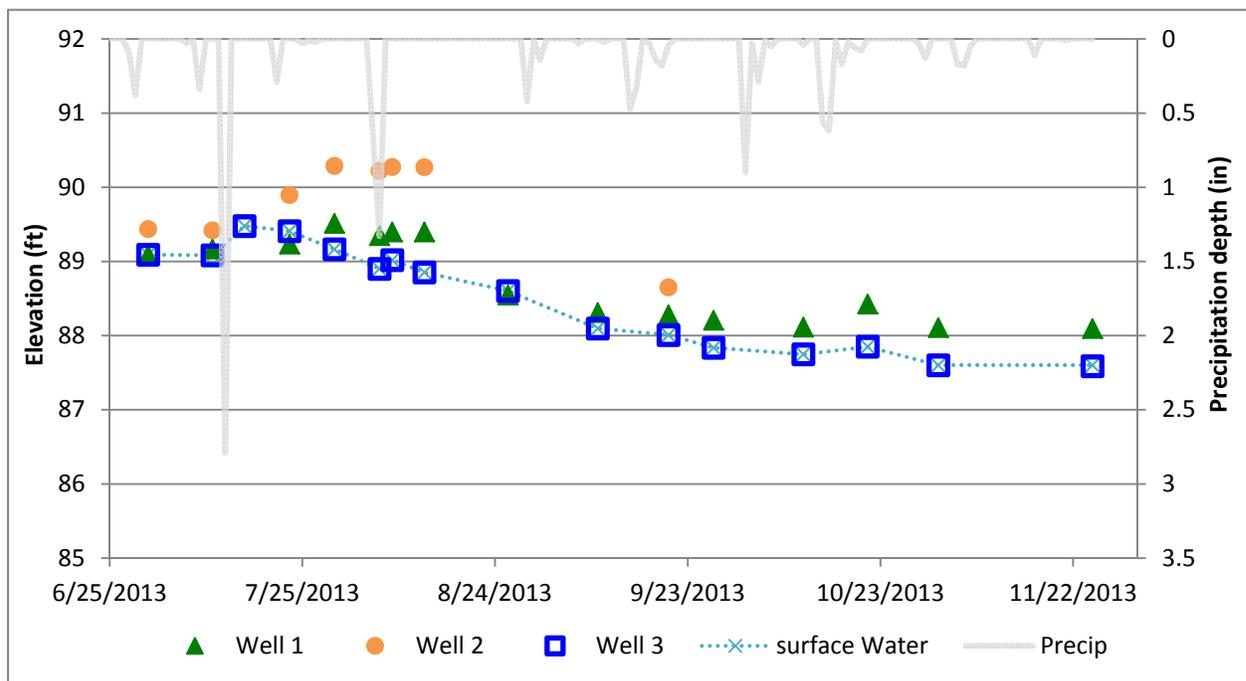
Figure 16. Groundwater piezometric head (Wells 1 and 2) and surface water elevation measurements (Well 3) at Utley Park, immediately downstream of Browndale Dam in Edina.
