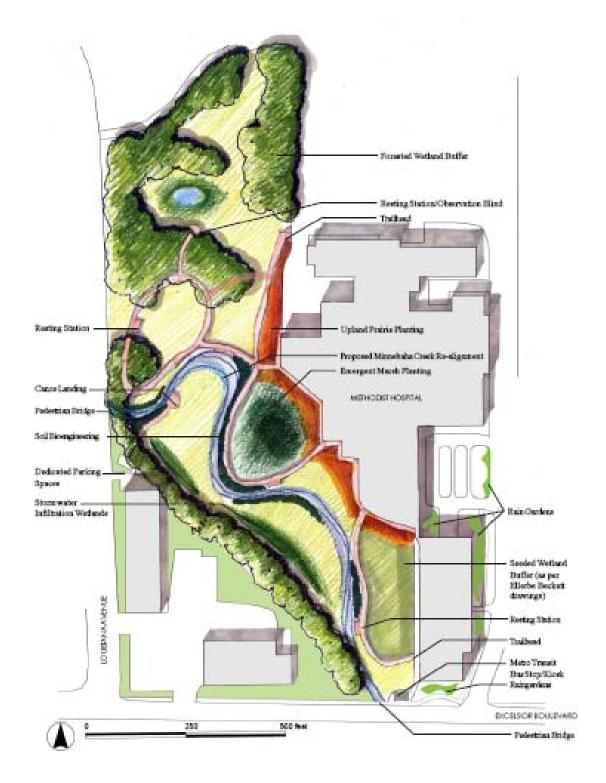
The project concepts included the restoration of a stream meander to the existing straight-line configuration of the creek, wetland vegetation restoration, construction of an elevated boardwalk and canoe landings to increase public access, and educational signage throughout the site.
